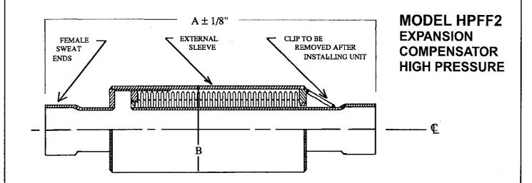
This expansion joint is designed for axial movement only. Pipe must be properly guided and anchored per the recommendations of the Expansion Joint Manufacturers Association.
