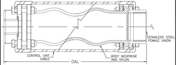
THIS FLEXIBLE JOINT SHOULD BE INSTALLED TO THE LENGTH SHOWN ON THIS DRAWING. THE CONTROL UNIT CABLES SHOULD BE REMOVED FOR THE INSTALLATION OF THE UNION ENDS. AFTER INSTALLATION THE CONTROL UNIT CABLES SHOULD BE REINSTALLED TO PREVENT MOVEMENT PAST DESIGN LIMITS. THIS PRODUCT IS NOT INTENDED FOR TORSION.
